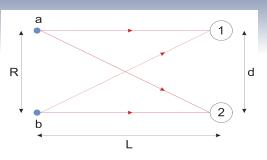
Intensity interferometry was discovered in 1950s by Hanbury-Brown, Twiss (HBT Interferometry) as a method of measuring the angular diameters of radio sources.
