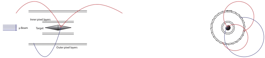
Figure 6.7: Minimum detector configuration for early commissioning with central silicon only (phase IA).
