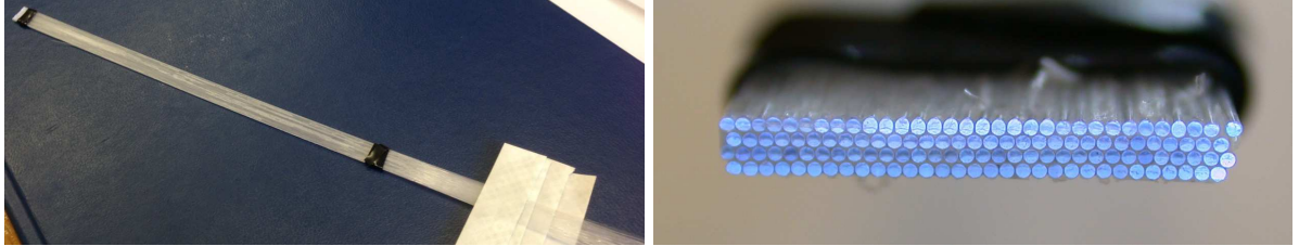
Figure 11.3: Photos of a Sci-Fi ribbon ( left ) and of its cross section ( right ). The uniform staggering of 4 Sci-Fi layers is clearly visible.
